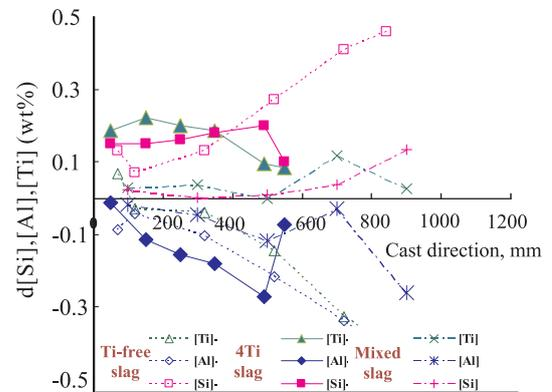
**Fig.3.** Effect of slag on [Al], [Ti] losses using: Ti-free slag 4Ti slag and mixed slag.
