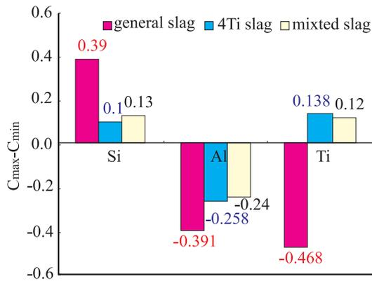
Fig.4. [Al], [Ti], [Si] variations for different slags.
