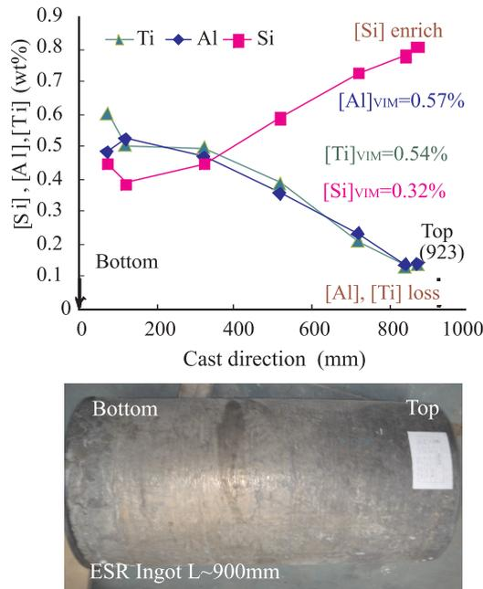
**Fig.1.** [Ti], [Al], [Si] fluctuated along axial direction of ESR ingot.
