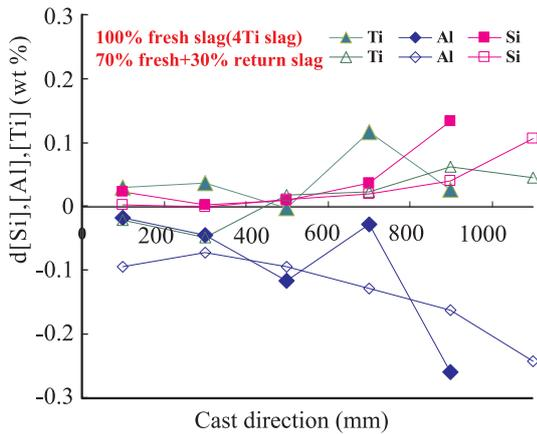
Fig.6. Returned slag shows a better control over [Al], [Ti], [Si].
