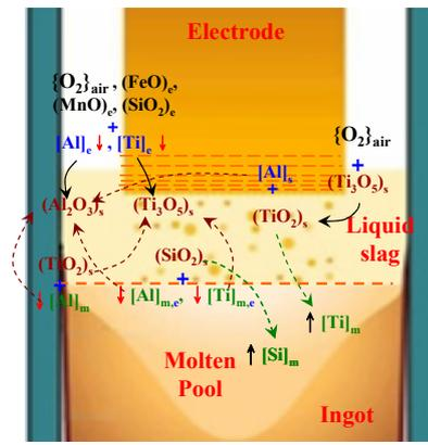
Fig.2. Schematic of the Al, Ti, burning loss and Si enrichment behavior during ESR process.
